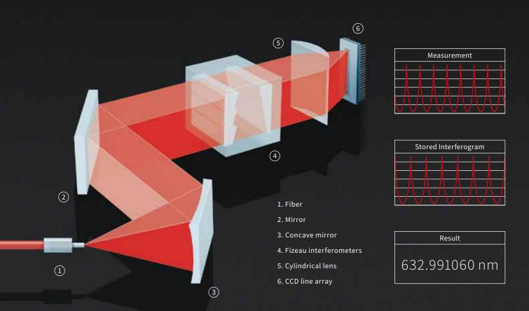
The light is coupled into the device via a fiber and then collimated by a mirror, before entering the solid-state Fizeau-interferometers. The interference pattern is imaged by a cylindrical lens onto CCD photodiode arrays. This recorded pattern is transferred to your computer via a high-speed USB connection which allows data acquisition rates of up to 50 kHz.
