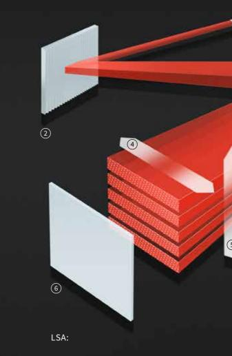
The LSA utilizes an echelle grating and a low order grating in two separate beam paths. The echelle grating provides the LSA with high resolving power, enabling high accuracy measurements. The first order grating makes it possible to overcome the wavelength indeterminancy of the echelle grating.
