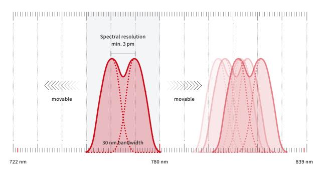
At any time, the measured signal has to be not wider than 30 nm, but this 30 nm window can be freely selected for each measurement shot inside the 15% measurement range (117 nm if centered around 780 nm).
