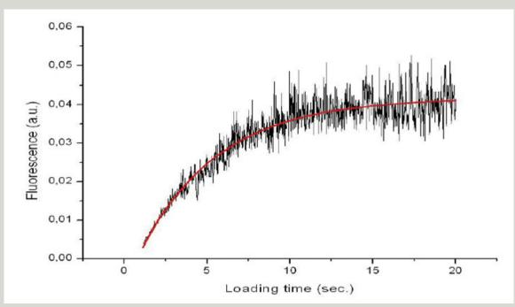
Loading a Magneto-Optical-Trap (MOT) with cold atoms. Laser frequencies of two DFB lasers are controlled by WS Ultimate-10. Fluorescence signal of cold Rb-atoms measured by a photodiode.
