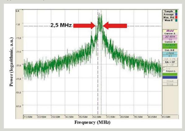
HighFinesse DFB laser diode controlled by WS Ultimate-10. Typical linewidth of the HighFinesse DFB laser < 2,5 MHz. High quality laser current and temperature controllers are available at HighFinesse.
